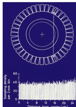
Fig. 12 An array of unequally spaced quad BGO detectors and its linear sampling density distribution of Positologica-II
