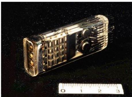
Fig. 19 A quad-PMT developed for SHR-1200
