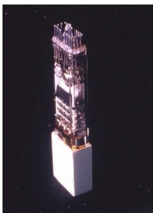
Fig. 20 A quad-PMT optically coupled with four BGO crystals
