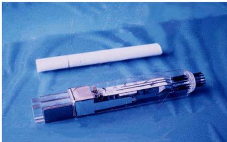
Fig. 15 A twin BGO detector developed for Positologica-IV
