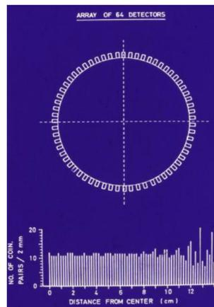
Fig. 7 An array of unequally spaced detectors and its linear sampling density distribution of Positologica-I
