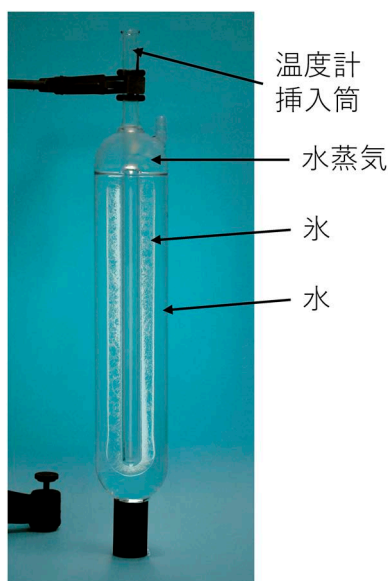
Fig. 2 Water triple point cell (photograph courtesy of AIST): liquid water, solid ice, and water vapor can coexist in a stable equilibrium. The tube in the center of the cell is used for calibration of thermometers
