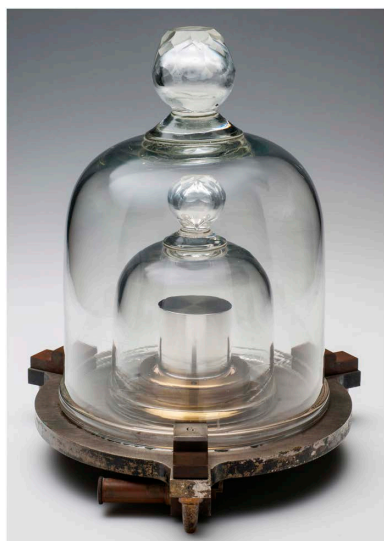
Fig. 1 The Japanese Prototype of the Kilogram (photograph courtesy of AIST)
