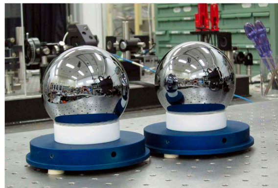
Fig. 5 Single crystals of silicon sphere (photo courtesy of AIST)
