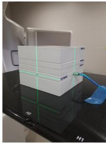
(a) Appearance of this audit for the photon standard dosimetry. The distance from the phantom surface to the mechanical center of the chamber is 10 cm.
