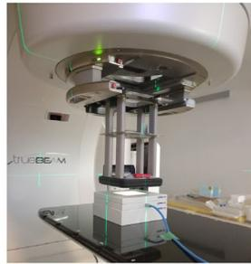
(b) Appearance of this audit for the electron standard dosimetry. The distance from the phantom surface to the mechanical center of the chamber is 3 cm.
