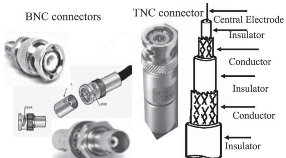
FIG. 4. BNC, TNC, and components of the triaxial cable.
